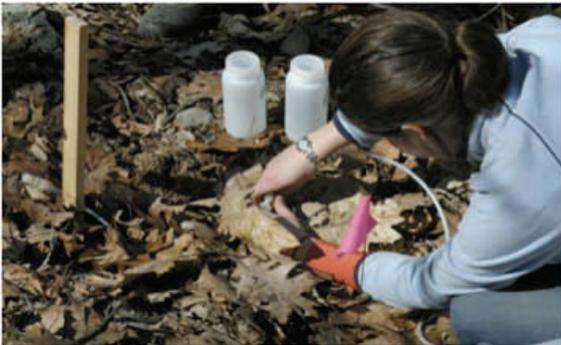
**Hannah Roth, a former Research Associate at the Forest, using a lysimeter to collect water that percolates through the soil into streams and groundwater so its chemistry can be analyzed to study nutrient cycling and possible water degradation.**
