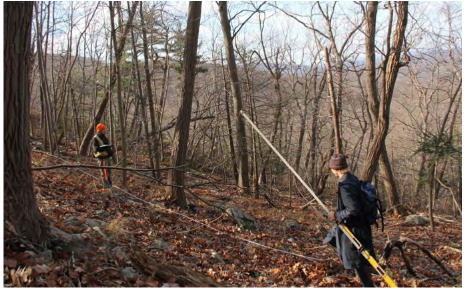
Eddie Walsh and Whitney Schuster obtaining side-slope measurements and identifying trees for removal. (Photo: Kate Terlizzi)
