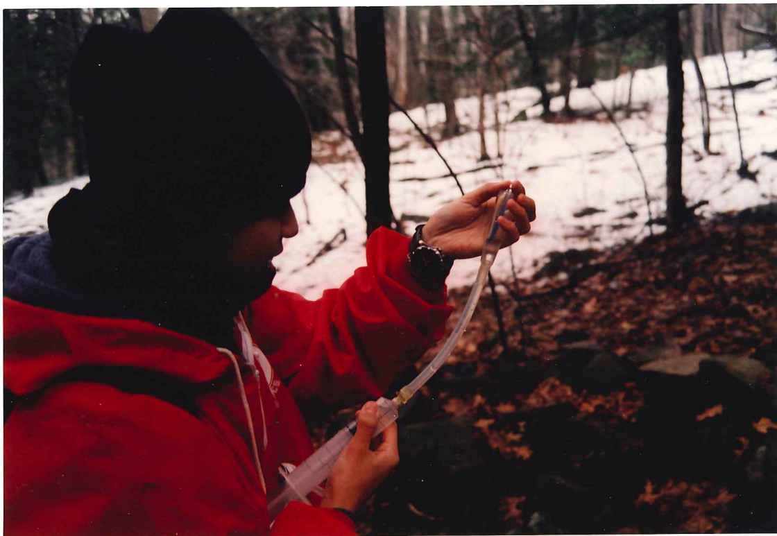
Sampling water from Frog Rock Spring with syringe, filter and bottle
