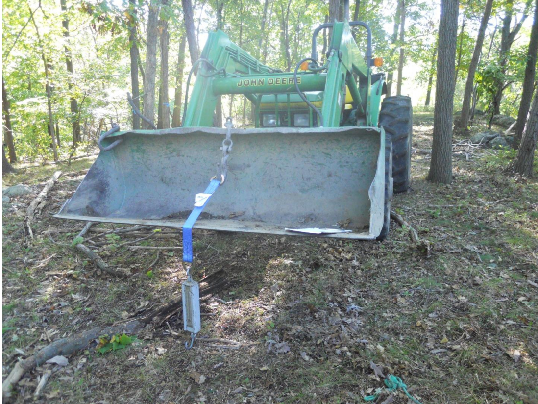
Figure 2. Tractor holding the scale used to measure felled trees. This picture shows the method of how the entirety of each tree is weighed. Each piece was suspended from the scale to get the tree wet weight.
