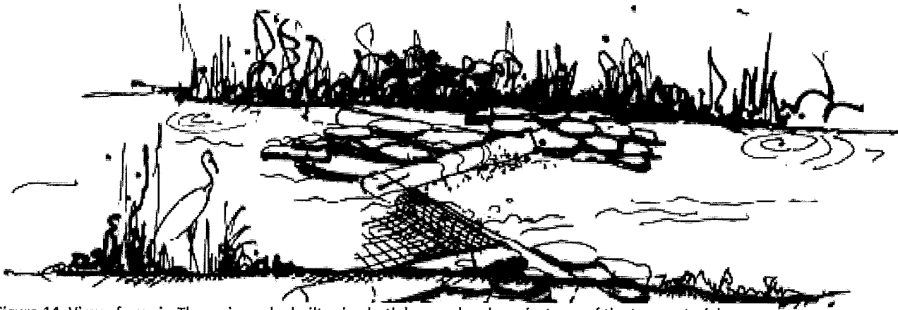
Figure 14. View of a weir. The weir can be built using both logs and rocks or just one of the two materials depending on the situation (Stream Corridor Restoration Handbook, 2010).
