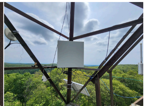
LEFT: Eastern painted turtle sunning itself; image credit: David Small. CENTER: Our GPS unit components include a rechargeable battery, a GPS component/antenna, and a GNAT asset tracker all connected via a circuit board; image credit Kristen Kallok. RIGHT: The gateway is attached to the supporting structure of the fire tower with a solar panel and 12-volt batteries for power. It can connect to the internet via a Wi-Fi connection to the wireless mesh network node at the fire tower; image credit: Kristen Kallok.
